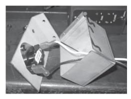
**14)** Reattach the thermodisc plate to the thermodisc cover using the 2 screws removed in step 10.
